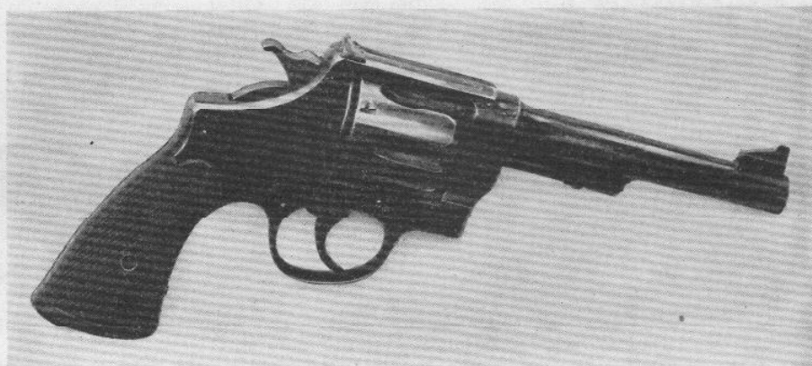
MODEL 1917 S. & W. FITTED WITH ADJUSTABLE TARGET SIGHTS BY W. H. BRADLEY
