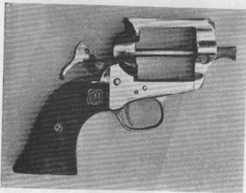
SINGLE ACTION FLAT TOP WITH REBOUNGING FIRING PIN, SPECIAL BASE PIN, AND GRIP SIMILAR TO CROFT GRIP EXCEPT CUT DOWN TO FIT A SMALL HAND. BASE PIN CATCH NOT YET FITTED. WORK DONE BY BRADLEY
